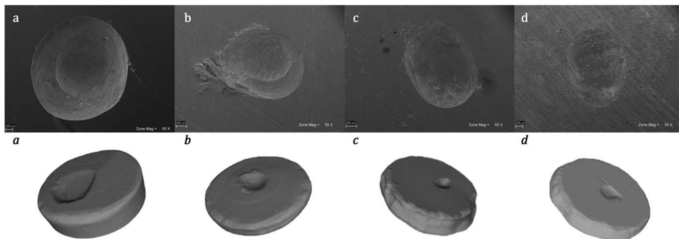
Figure 2 Scanning electron microphotographs (upper row; original magnification 55 $\times$ ) and three-dimensional meshes (lower row) showing the wear facets of some representative samples from the Filtek XTE heat-cured group (a), Aurocast8 gold alloy group (b), HRi-Function heat-cured group (c), and Imagine PressX glass-ceramic group (d).
