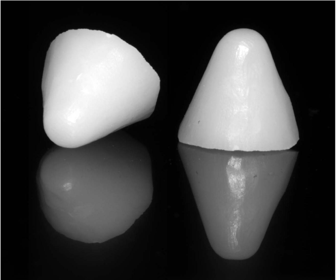
Figure 1 Standard zirconia cusps used as abrasers in the chewing simulation test.
